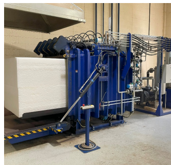
Fig 1: Reticulation Chamber with two polyurethane buns to be reticulated
