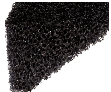
Fig 2: Reticulated Polyurethane Polyether Foam, approximately 30 PPI
