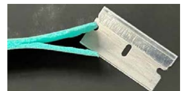
Figure 5: End of sample skived using razor
