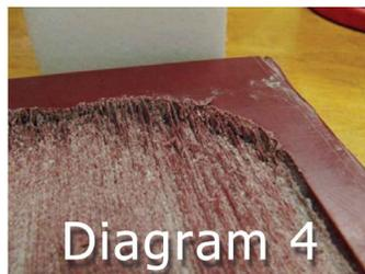
It is very important that the space inside the die is large enough to hold the ejection material and the material to be cut. The cutting press needs to compress the material to be cut so the edge of the cutting blade can reach the cutting surface. This will increase the cutting force requirements to the point that a cut cannot be made. The compression of foam can take the cutting force requirements off the charts. With proper die-making, these problems can be taken off the table.
