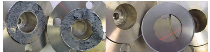
Picture: Flange sticking of a standard graphite gasket vs graphite gaskets with inerted surface treatment
